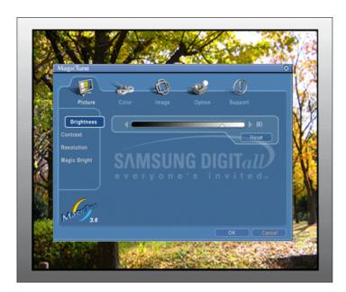
The OSD mode makes the adjustment of settings on all monitors easy. When selected , each tab on top of the control window displays the general descriptions of the sub-menu items for adjustment.
